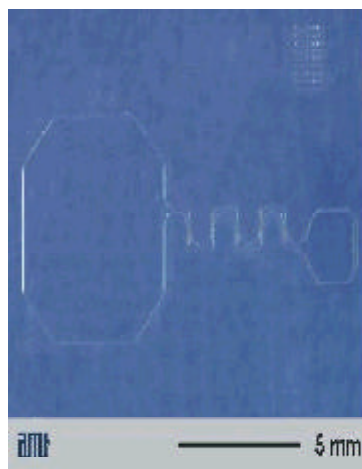
Figure 1 Plastic microchip for in vitro fertilization fabricated by Jenoptik (Jenna, Germany) (mikrotechnik@jenoptik.com) (channel at the left contains eggs and is connected via 100 um wide sperm selection microchannel to the semen chamber.
